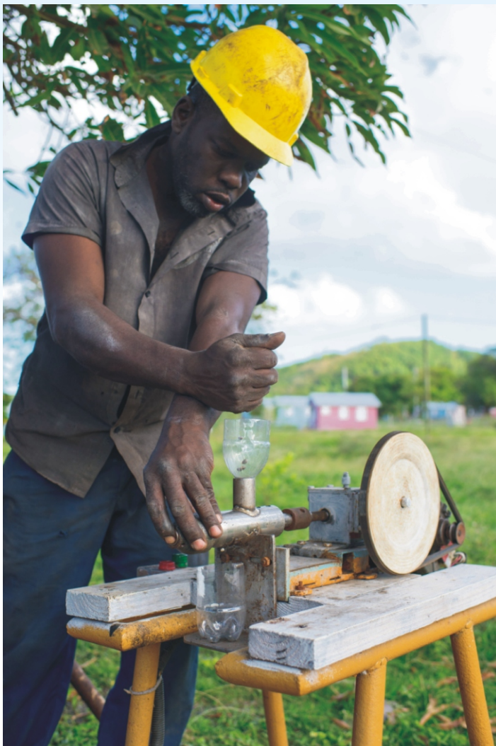
Mr. Stephen Whinn pours oil nuts into the machine. The result will be cold pressed castor oil.
